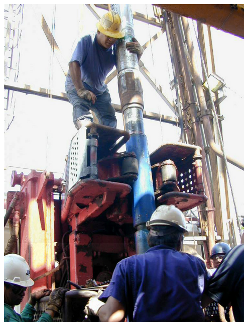
Assembly of the ADN tool aboard the JOIDES Resolution.
