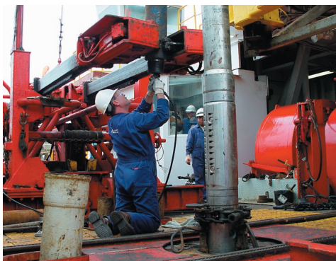
Assembly of the RAB Coring Tool aboard the JOIDES Resolution .
