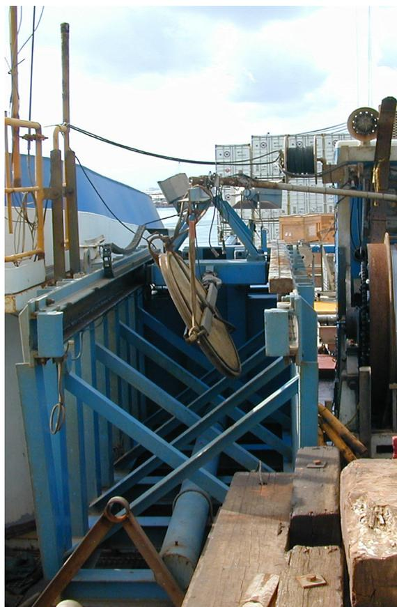
Wireline Heave Compensator (WHC) as installed on the JOIDES Resolution.
